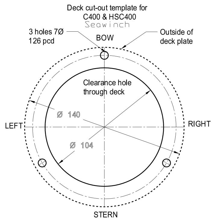
Standard studs will suit decks up to 30mm thick M6 extended studs can be supplied to order Stiffen light construction deck with hard wood packer under-deck if necessary
